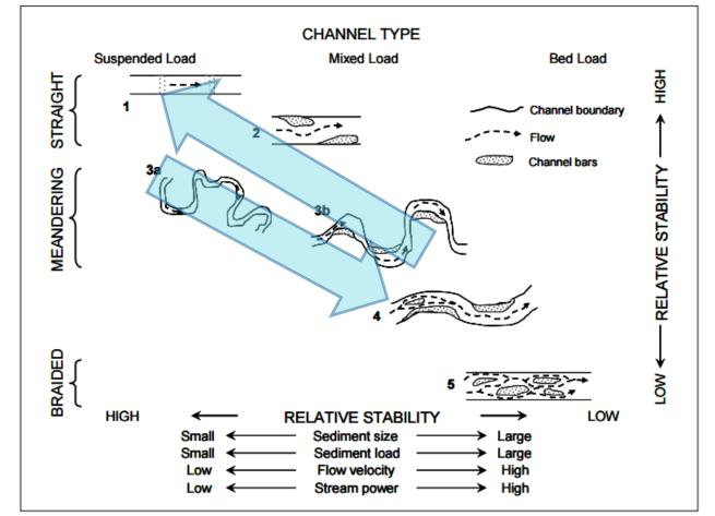
Figure 13. A qualitative classification of stream channels based on pattern (straight, meandering, or braided) and type of sediment load, along with flow and sediment variables and relative stability with regard to average erosional activity. From Schumm (1981).
