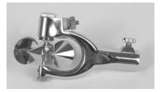
For use on stream channels with depths greater than 3 inches (~ 8 centimeters) and velocities greater than 0.1 feet per second.
