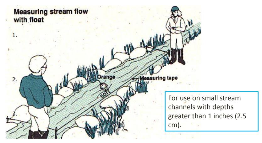
Because surface velocities are typically higher than mean or average velocities  $V_{mean} = k V_{surface}$  where k is a coefficient that generally ranges from 0.8 for rough beds to 0.9 for smooth beds (0.85 is a commonly used value)
