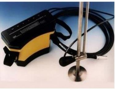
For use on stream channels with depths greater than 3 inches (~ 8 centimeters) and velocities greater than 0.01 feet per second.
