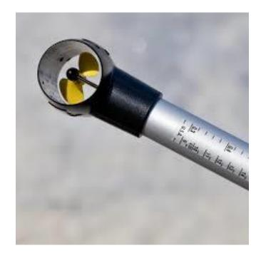
For use on stream channels with depths greater than 3 inches (~ 8 centimeters) and velocities greater than 0.1 feet per second.
