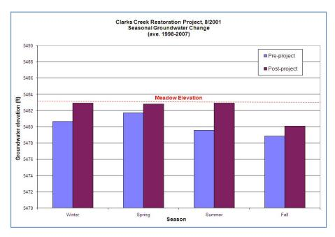
Figure 5. Seasonal average groundwater elevation changes from a pond and plug project on Clarks Creek in the upper Feather River watershed (unpublished monitoring data).
