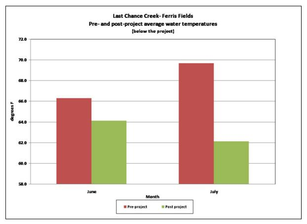
Figure 8. Summer water temperature change and below a pond and plug project at the Ferris Flat reach of Last Chance Creek.
