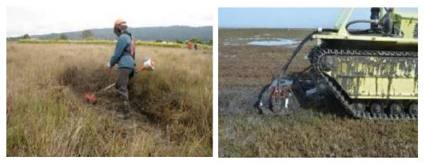
Image 2-1 – Representative Vegetation Removal Equipment. Handheld brushcutter (left) used to remove above-ground vegetation. Marshmaster (right) used to mow larger areas and grind (via rototiller) dense-flowered cordgrass rhizomes. Photo credit: A. Pickart (USFWS 2017)
