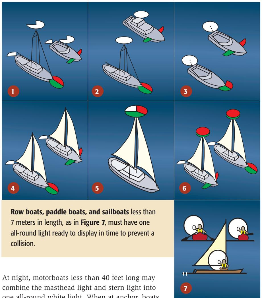
**Row boats, paddle boats, and sailboats less than 7 meters in length, as in Figure 7, must have one all-round light ready to display in time to prevent a collision.**
