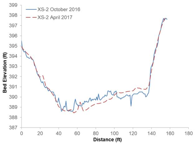
Figure B-9. XS-2 bed elevation profiles before and after the 2016-2017 winter storms.
