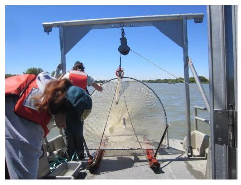
*Figure 3. The townet in the field ready for deployment. Note flowmeter in center of net mouth with CB net attached on top of the D-ring frame.*
