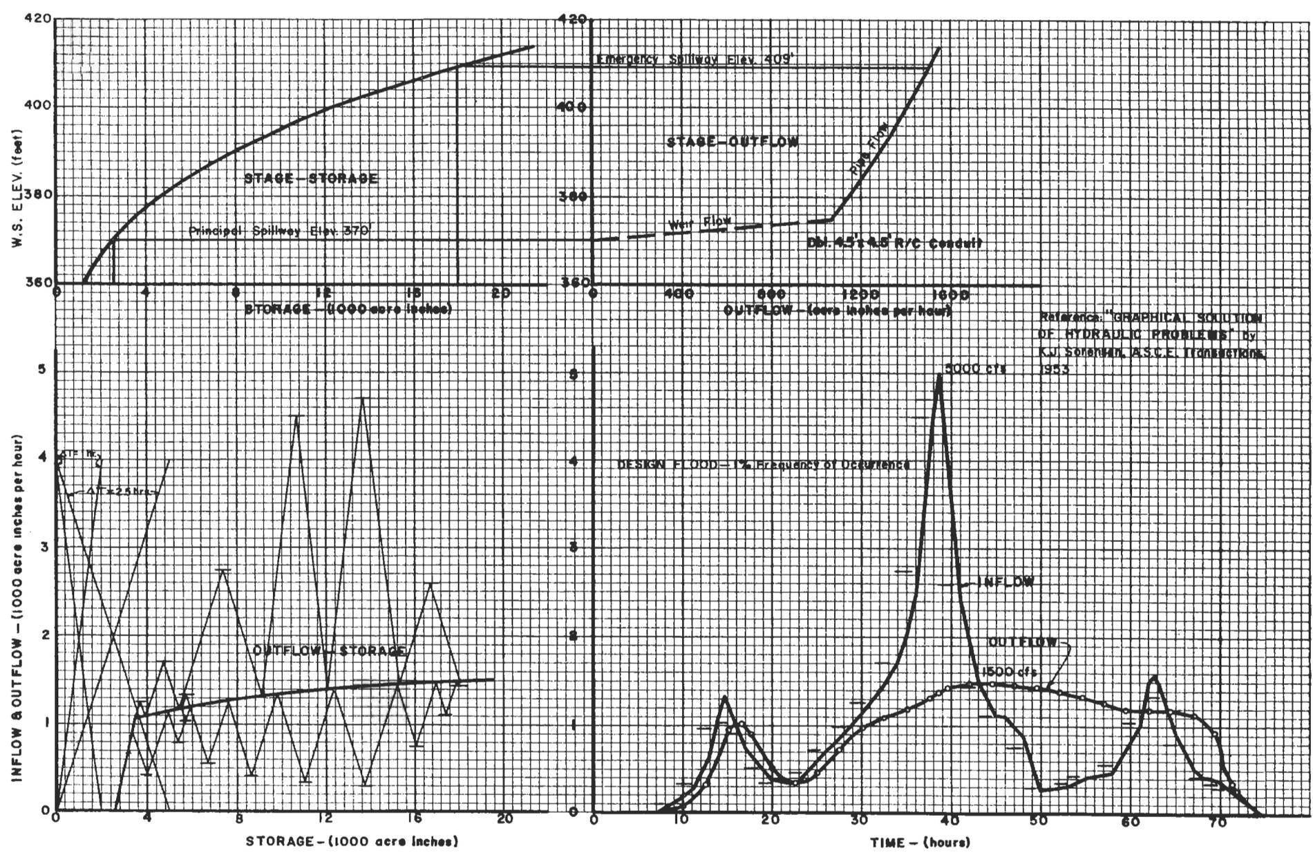
FIG. 9: Flood Routing: MATANZAS CREEK RESERVOIR - Design Flood
