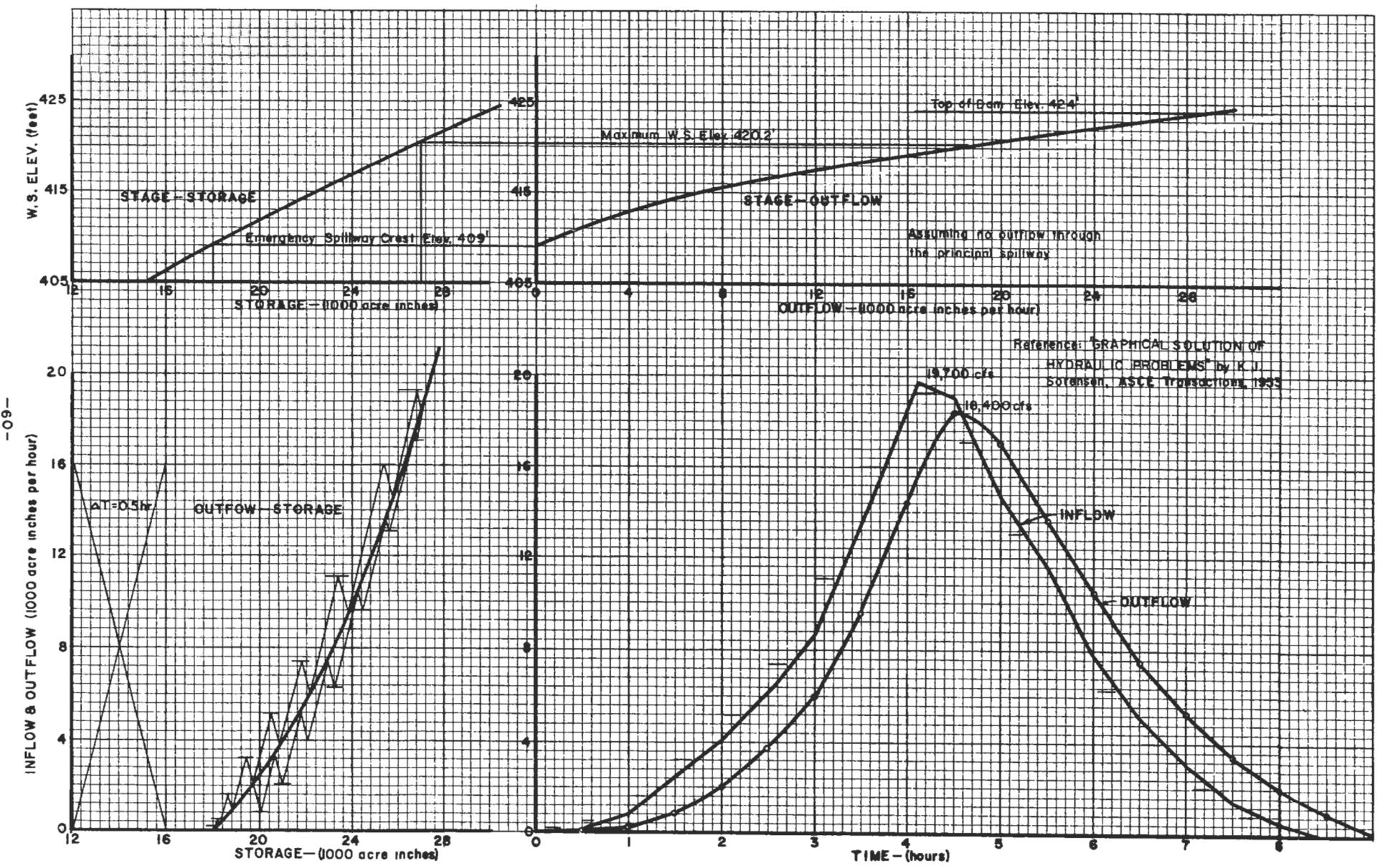
FIG. 11: Flood Routing : MATANZAS CREEK RESERVOIR - Emergency Spillway
