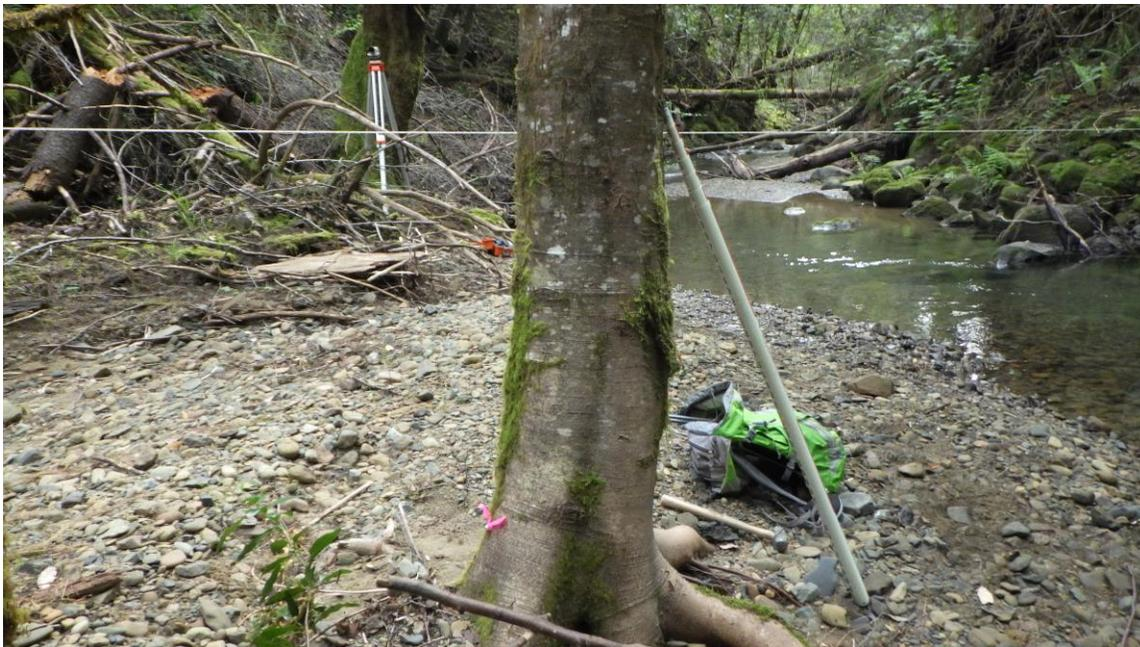
**Figure 3.** Vertical benchmark driven into the base of tree trunk marked with flagging tape in foreground, and auto level in background.
