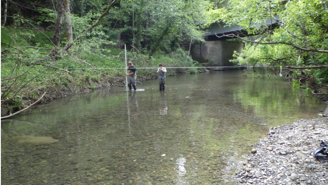
**Figure 4.** Measuring WSEL and velocity along transect LRT62 in Lower Redwood Creek reach.
