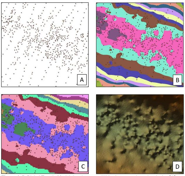
**Figure A-5.** Digital Terrain Model development: (A) bed topography points in ArcGIS; (B) shapefile converted to raster (Topo to Raster); (C) GeoTIFF; and (D) Terrain layer in HEC-RAS.
