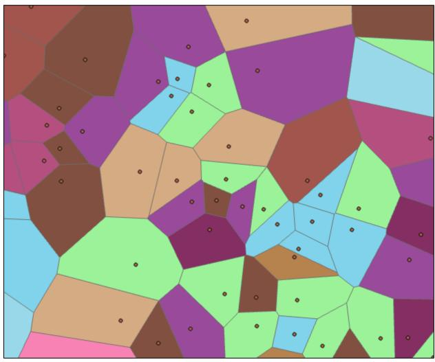
Figure A-3. Point values converted to Thiessen polygons.
