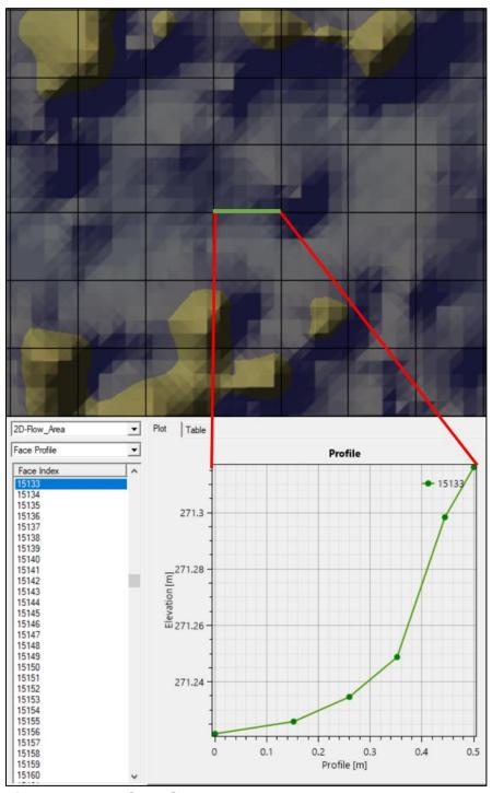
**Figure A-8.** HEC-RAS sub-grid bathymetry, looking down on a portion of the wetted channel from above. The green line is a flat cell face, but considers the varied terrain below shown by the elevation profile. The number 15133 is the reference for the cell face in the model.
