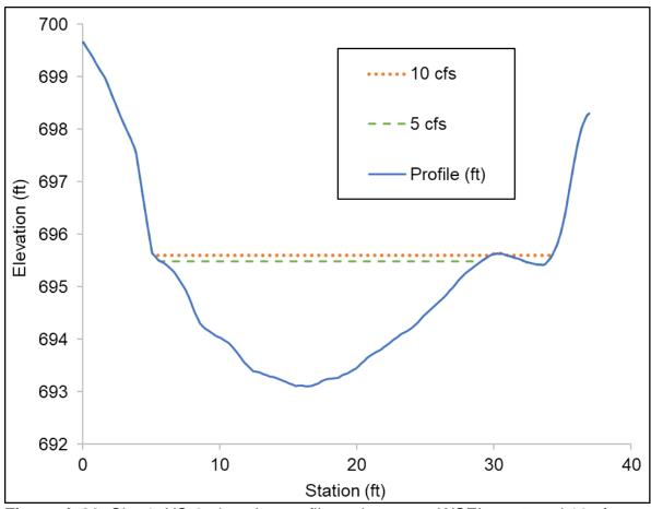
Figure A-33. Site 1, XS-2 elevation profile and average WSELs at 5 and 10 cfs.
