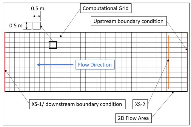
Figure A-6. HEC-RAS 2D model components.
