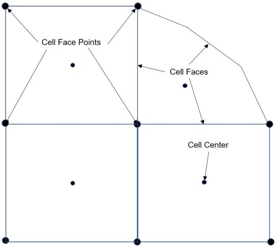
**Figure A-7.** Close-up view of four HEC-RAS computational grid cells including one irregular shaped boundary cell. The figure indicates which parts of the grid are cell faces, cell face points, and grid cell centers.
