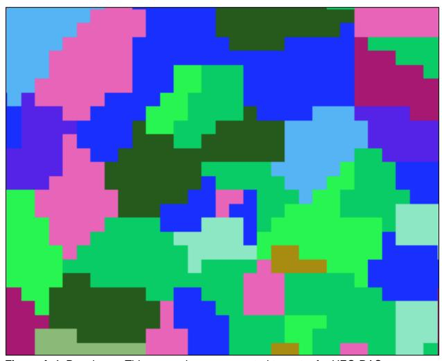
**Figure A-4.** Roughness Thiessen polygons converted to raster for HEC-RAS.
