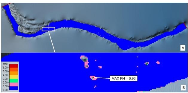
**Figure A-17.** (A) Site 1 FN display at 30 cfs. Blue cells are FN <1.0, purple, green, and red cells appear sporadically near bed, bank, and substrate boundaries where FN >1.0. (B) Zoomed in on cell with max FN.
