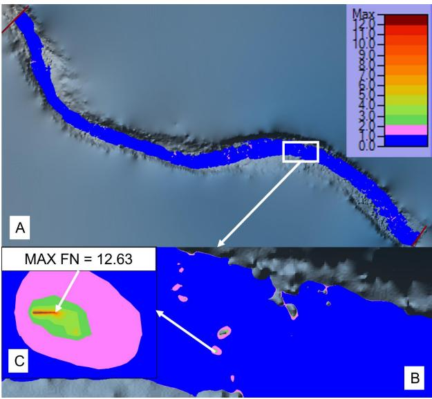
**Figure A-18.** (A) Site 2 FN display at 70 cfs. (B) Blue cells are FN <1.0, purple, green, and red cells appear sporadically near bed, bank, and substrate boundaries where FN >1.0. (C) Zoomed in on cell with max FN.
