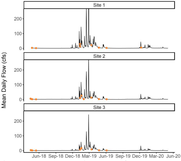
**Figure A-1.** Flow time series developed for each study site. Orange markers indicate when flow-WSEL data were collected. The peak flow at Site 1 on February 27, 2019, was estimated to be above 2,000 cfs.
