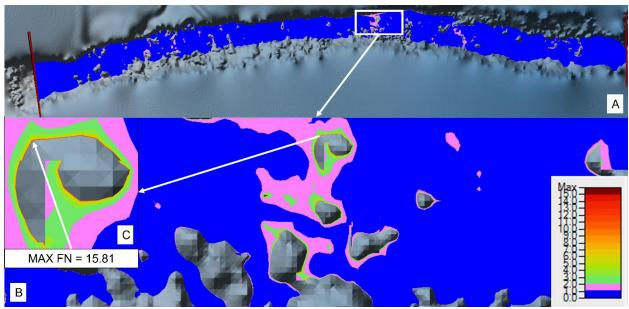
**Figure A-19.** (A) Site 3 FN display at 17 cfs. (B) Blue cells are FN <1.0, purple, green, and red cells appear sporadically near bed, bank, and substrate boundaries where FN >1.0. (C) Zoomed in on Max cell FN.
