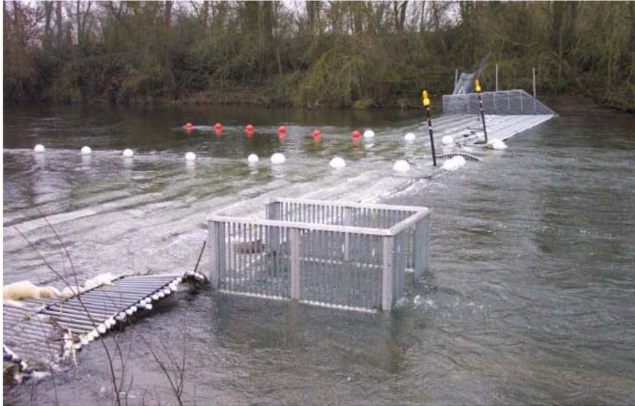
**Figure 6.** Resistance board (Alaskan style) weir with a Vaki Riverwatcher System on the Stanislaus River, CA. Photo credit: David Hu, USFWS.
