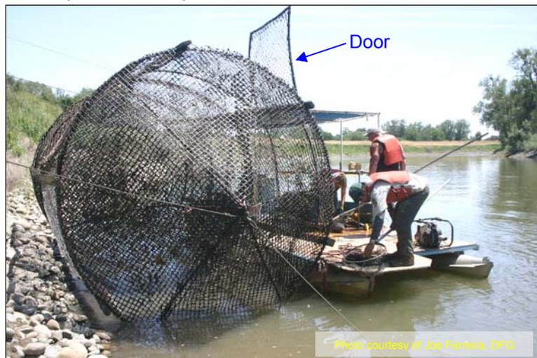
One of two methods was used to roll the traps up and down the riverbank: a cable-and-block system or an electric winch. When the trap and boat were in position, fish were netted from the trap and tagged on board the *Kayot*.
