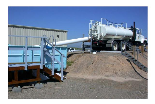
Figure 5 Fish truck backed up to the release pipe and ready to release fish from a CHTR trial into the release pool after a simulated fish haul
