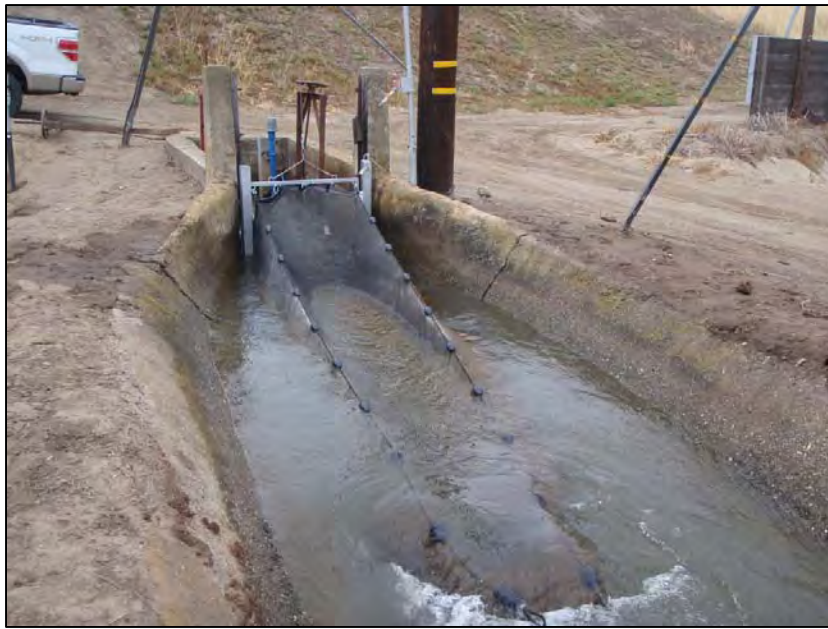
Figure 13. The fyke net and associated apparatus used to sample for fish entrainment in the Cranmore trapezoidal concrete canal.
