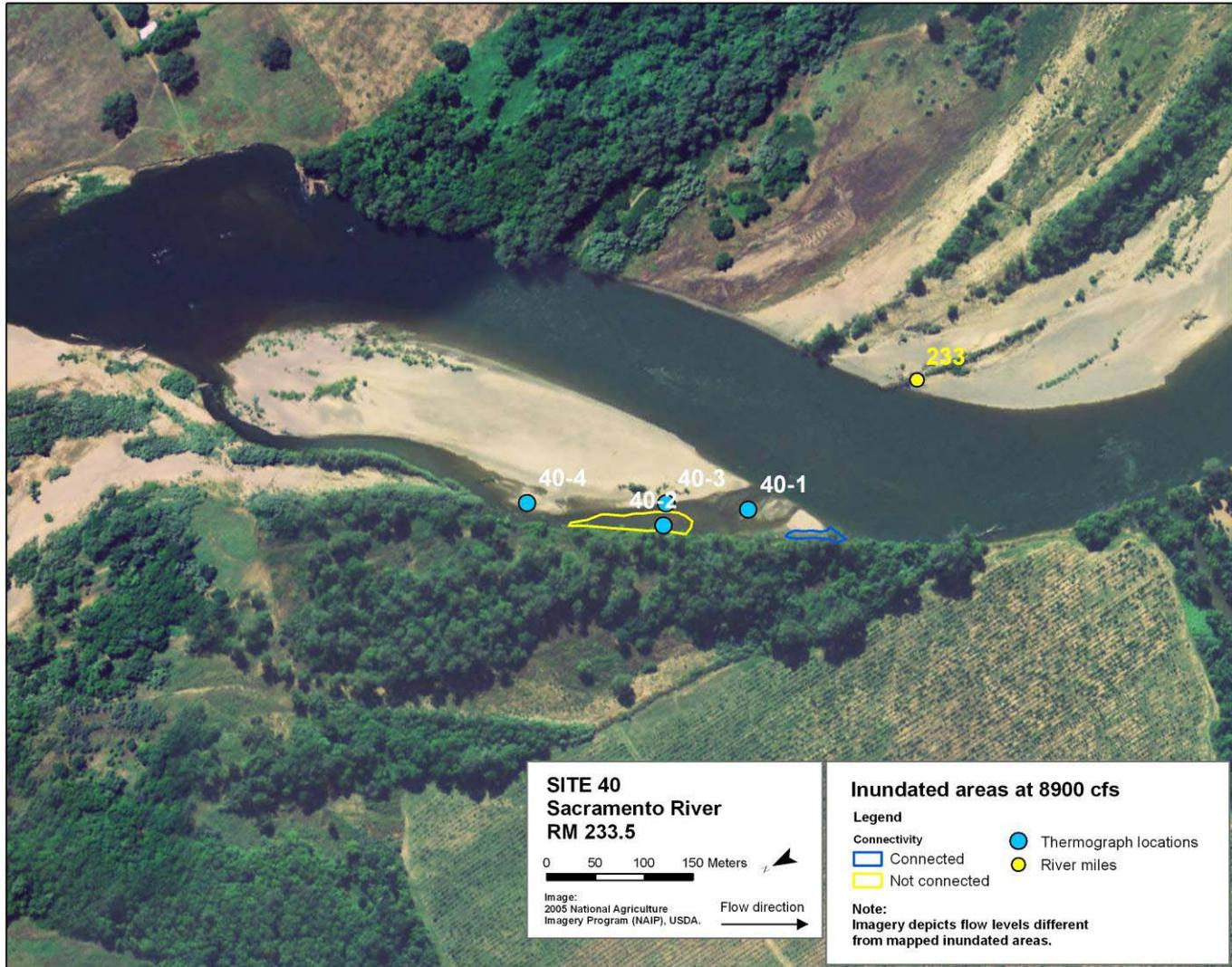
**Figure 47a.** Inundated areas of site 40 (RM 233.5R) at flows of 8,900 cfs , areas observed and drawn during field mapping.
