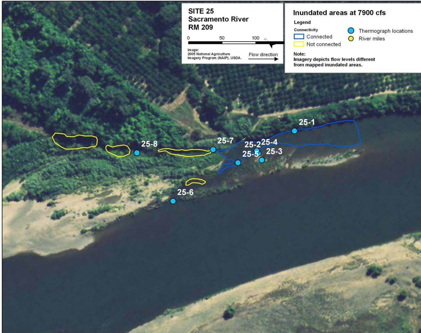
**Figure 34a.** Inundated areas of site 25 (RM 209L) at flows of 7,900 cfs, areas observed and drawn during field mapping.
