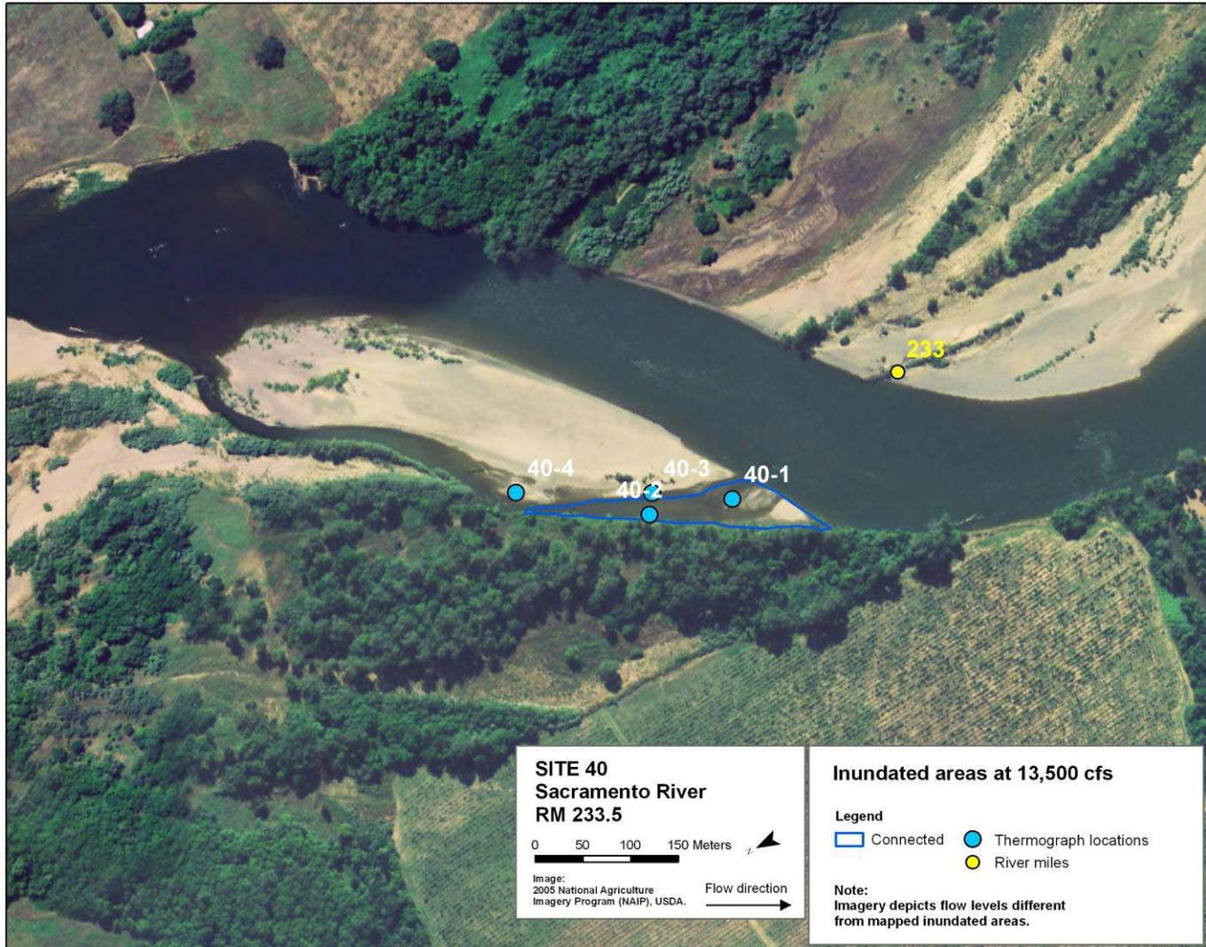
**Figure 47b.** Inundated areas of site 40 (RM 233.5R) at flows of 13,500 cfs , areas based on thermograph temperature records and field surveys.
