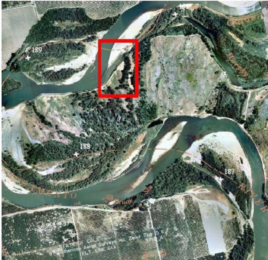
**Figure 2.** Example of a scour channel that forms on the downstream end of a point bar, providing seasonally inundated, shallow-water habitat that can support rearing of salmonid fry. (Photo Source: CDWR 1999)
