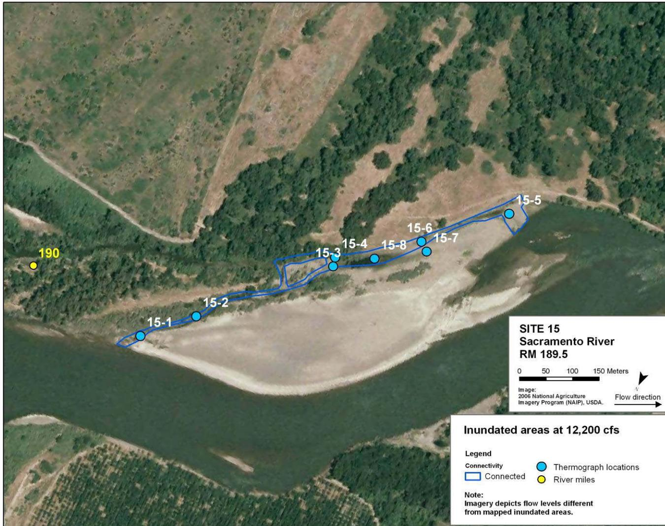
**Figure 24d.** Inundated areas of site 15 (RM 189.5L) at flows of 12,200 cfs , areas based on thermograph temperature records and field surveys.
