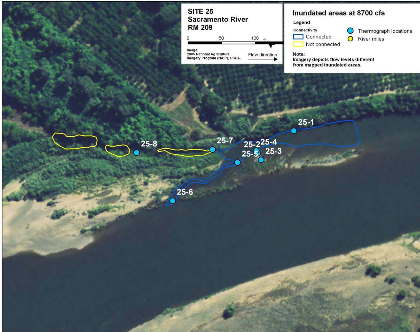
**Figure 34b.** Inundated areas of site 25 (RM 209L) at flows of 8,700 cfs, areas observed and drawn during field mapping.
