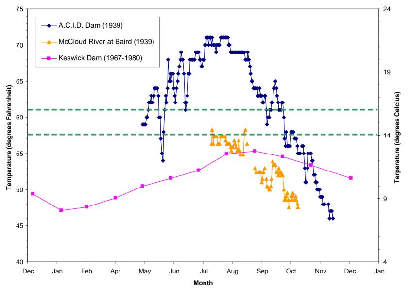
Figure 4.2-11. Temperatures at A.C.I.D Dam and the McCloud River at Baird and below Keswick Dam (1967-1980 average). Temperatures below 57°F (14°C) generally allow for high survival of incubating eggs and temperatures above 61°F (16°C) result in mortality.
