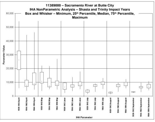
Figure 2-6. Comparison of mean monthly discharge at the Butte City gage for three time periods (see Figure 2-5 for explanation of time periods and box and whisker plots). Note the "flow reversal" pattern with increased average monthly flows under regulated conditions in summer and reduced flows in winter months. Source: CDWR 2001, as reported in TNC 2003.
