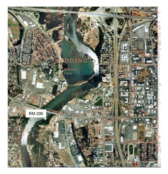
Figure 2-2. Lasting effects of aggregate extraction. Kutras Park (center) was one of the primary sources of aggregate for construction of Shasta and Keswick dams. Overall, more than 7 million cubic yards of sediment has been mined from the upper Sacramento River basin. Much of the mining has been done on the mainstem channel and floodplain. Remnant mining pits can trap sediment and disrupt the continuity of bedload transport. (Source: CDWR, 1999. Sacramento River Aerial Atlas.)
