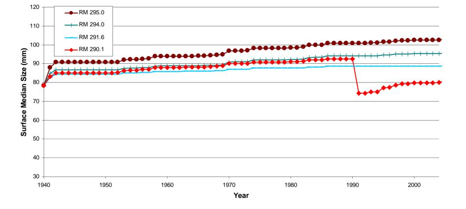
Figure 4.2-22. Simulated surface median size at four locations on the Sacramento River, beginning with a D50 of 78.4 mm (3.09 in). Using the TUGS model, we conducted a sensitivity analysis to assess the effects of a different initial grain size on bed coarsening. The results suggest that the grain size to which the bed will eventually coarsen is relatively insensitive to differences in the initial grain size.
