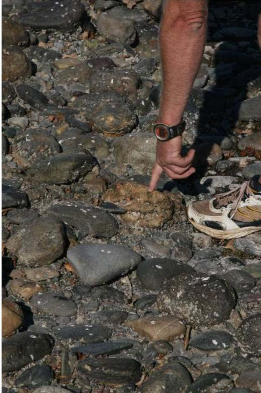
Figure 51. Painted rock in one of 3 scour boxes at SW-6 (RM 271.7). Only a scant residue of paint remains on rocks in each box. This suggests that significant abrasion has worn it away during high flows. The fact that the rocks are still in the scour boxes, 20 m apart as they were the year before, nevertheless implies there has been minimal disruption of the bar surface.
